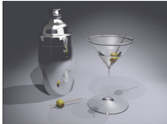
Same scene rendered with higher sampling shows smooth edges. Sampling range: 1 to 16
